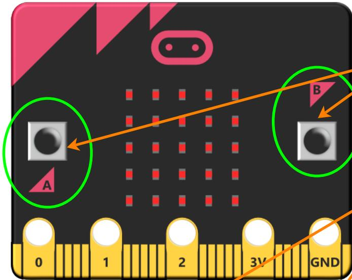
The BBC micro:bit has quite a few ways of interacting with it, however, most obvious are the clearly labelled A and B buttons on the front.
